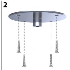
Fix the base on the ceiling by screwing it into dowels. (Fixing screws are not provided)
