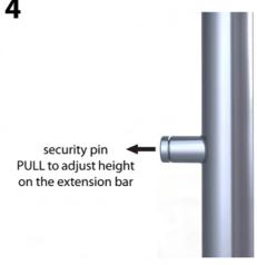
Adjust the height of the extension bar system by pulling the security pin on the side and raising or lowering the bar.
