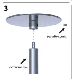
Screw in extension bar system into base and secure it with the side security screw.
